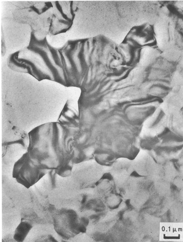
Figure 13 Hot-stage result of temperature increase from room temperature to 350°C in 40 min.
